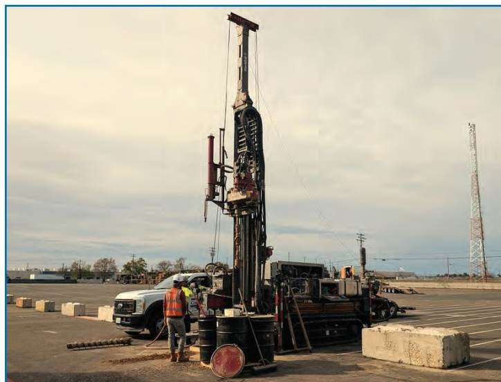
Air Force environmental contractors using a drilling rig to do geotechnical soil sampling at an Old Magpie Creek Channel project site. Results from the soil sampling at these sites will help with upcoming soil excavation work.
